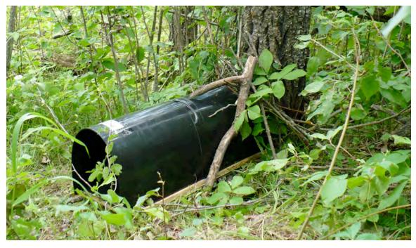
Figure 5. Metal plate component of the track plate used in the American marten Turtle Mountains study during the summer of 2007. The dark end is covered with soot from an acetelyne torch. The white paper is household shelf liner paper placed sticky side up. The small length of metal showing at the end is where I placed the beaver meat and approximately 8 g of beaver castor.
