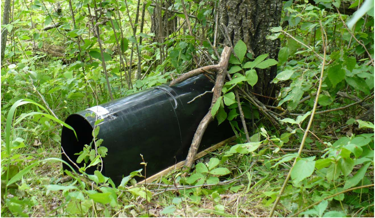
Figure 4. Track-plate-box used to survey for American martens in the Turtle Mountains of North Dakota
