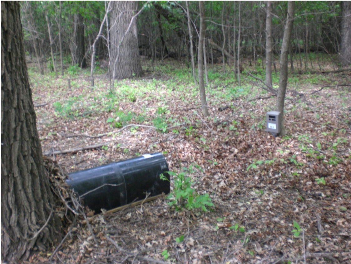
Figure 4. Track-plate-box and remote camera placed at survey sites in eastern North Dakota (2008, 2009) to detect fishers.
