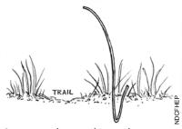
9-gauge wire used to make a support system for a cable loop.
