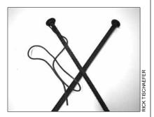
Re-rod stakes used to cross stake for anchoring. Support wire is welded to one stake to provide a system to support the cable loop.
