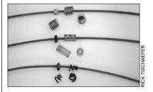
Various examples of support collars. Top to bottom: wire wound collar, plastic tubing, and twist-on collar.
