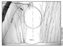
The 12 inch loop stop provides a reference point to the support collar. Placing the support wire in the support collar approximately 4 inches from the 12 inch loop stop will provide the desired 10-inch loop for catching coyote.
