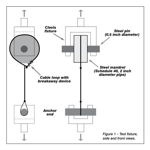
the peak load at which the cable device loop disassembles. Both methodologies make use of the same test fixture design to secure the cable loop.
