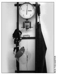
Personal protective equipment like safety glasses, face shield, gloves, and apron are worn while testing cable device breakaways.
