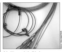
A baking soda boil helps remove the shine from new cable and components.
