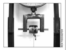
The mandrel (steel cylinder) and support frame for testing cable devices. A one half inch cold rolled steel rod holds the mandrel to the frame. Cold rolled steel rod is used because it will handle the stress of the pull without bending.
