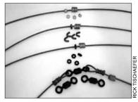
A variety of components can be used to make a loop stop. Top to bottom – aluminum ferrule, addon "c" stop, heat treated steel nut. and in-line swivel.
