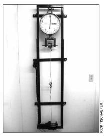
A battery operated winch driven pulling device. The double dial scale records the weight when the loop disassembles.
