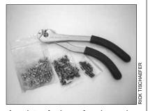
A variety of release ferrules and hand swagger to apply the ferrule to the cable end.
