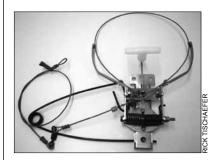
A Collarum spring powered cable device system. The entire device is fastened and covered (much like a foothold trap) and bait is placed on the white plastic "T". The coyote bites and pulls up on the plastic "T", causing the spring arm to throw the cable loop around the coyote's neck.
