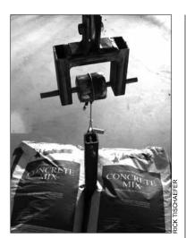
A static weight testing assembly using 5 – 60# bags of dry mix concrete for known weight. A platform was built with a center stem – the bags of cement are placed on the platform and a stem to connect the cable device for the test. This test is conducted by raising the mandrel with a rafter mounted electric winch.
