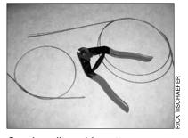
Good quality cable cutters are required to release incidental catches. Cut the cable loop, not the cable between the loop and the anchor.
