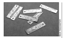
Trap tags made of copper or brass are inexpensive and will provide many years of service.
