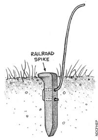
A railroad spike is used to provide a support wire in frozen ground. Re-rod can also be used for the same purpose.
