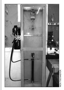
A testing device machine used by the North Dakota Game and Fish Department. A hydraulic ram pulls the cable and a digital scale with memory records the weight of pull. A plexiglas enclosure protects the operator from flying components when the loop disassembles.
