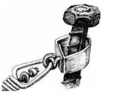
These two swivel combinations can be used for anchoring a restraining cable device. If you are using a single re-rod stake, make sure it is long enough to anchor your equipment properly.
