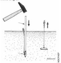
Earth anchors work well as an anchoring device for cable devices when soil conditions allow.
