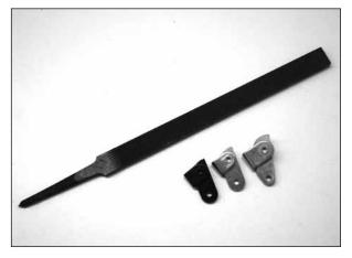
Cam locks can be purchased with and without teeth. A cam lock file is used to create or repair teeth on these locks.
