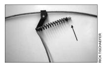
An example of a release ferrule breakaway device.
